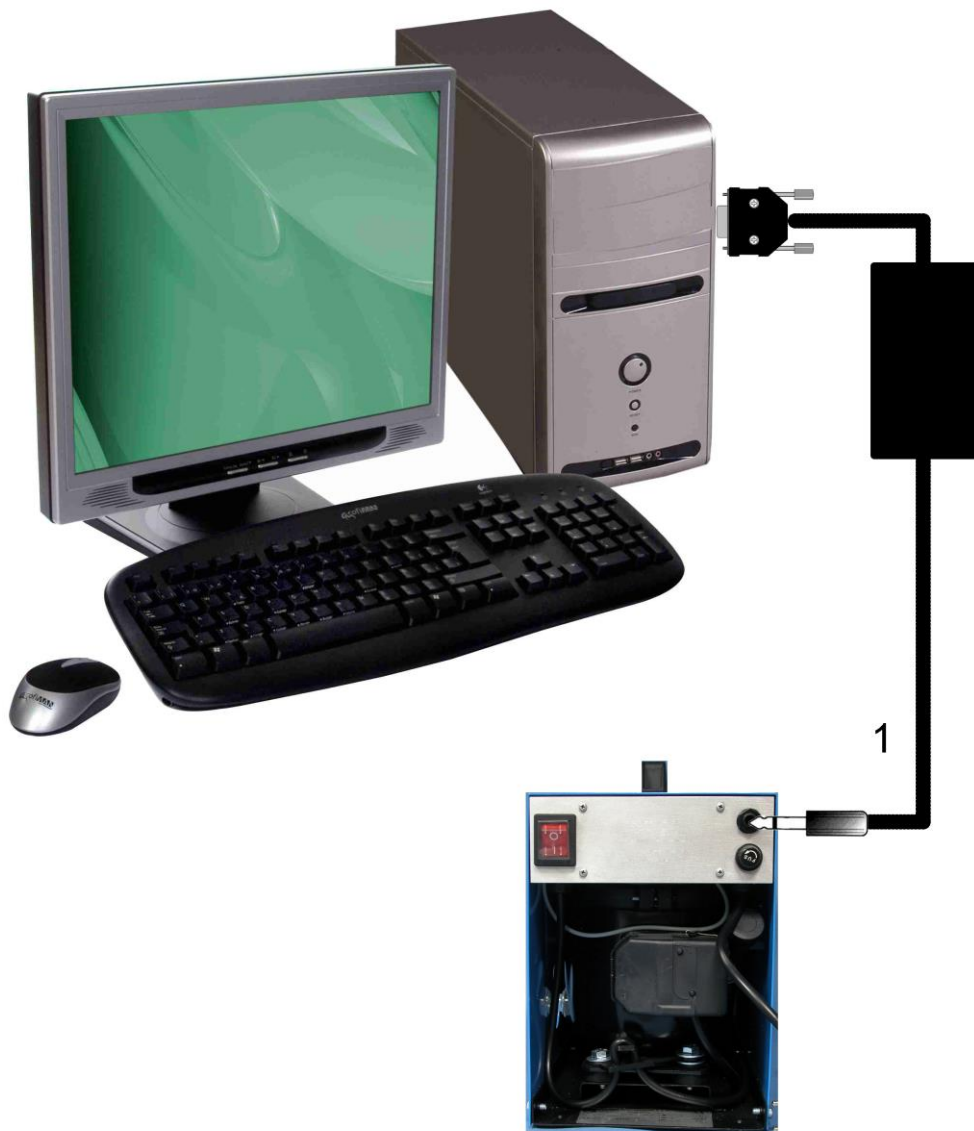
Figure 8. Connecting the SMART cable to the jack connector.
